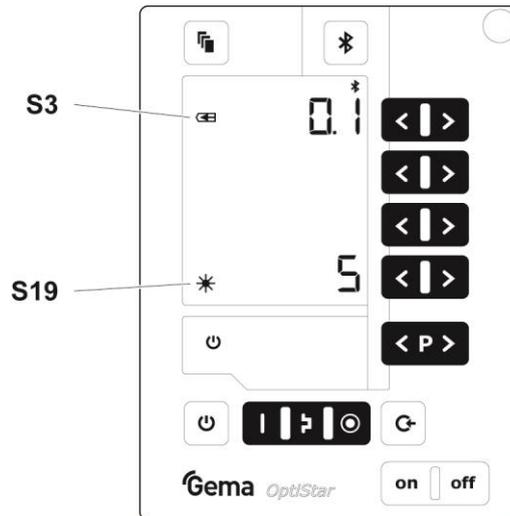
fig. 10: Displays and LEDs, Level 2
