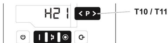
The help codes are stored in an error list in the order of their appearance. Each error in the list must be individually acknowledged with the keys **T10** or **T11**.
