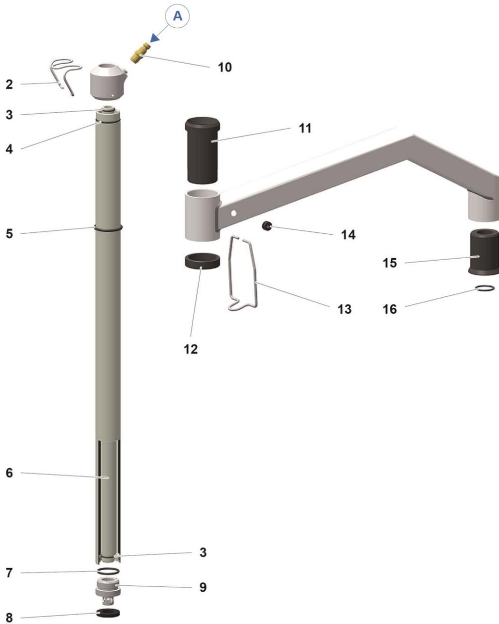
fig. 18: Fluidizing/suction tube – spare parts
